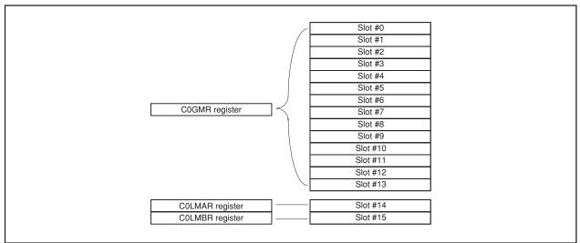
Figure 18.17 Correspondence of Mask Registers to Slots
